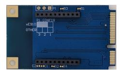
The XBEE-EVB-ADAPTOR has been designed to plug into the MPCI connector on board to allow for interfacing with XBEE carrier boards.
