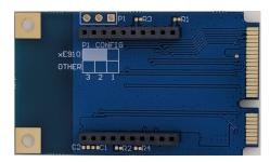
To allow for interfacing of the XBee footprint on the existing carrier board, an adaptor board from XBee to MPCI is available. Part number - XBEE-EVB-ADAPTOR.
