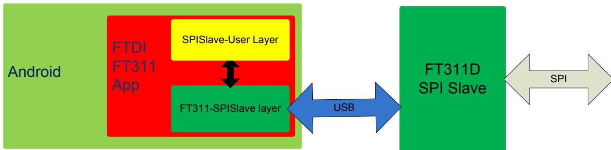
Figure 7.1 : Android FTDI FT311D SPI Slave Application
