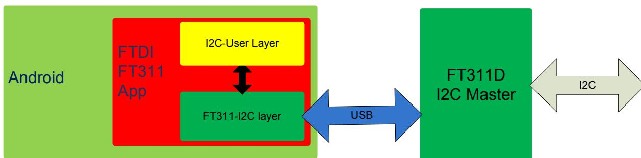
Figure 5.1 : Android FTDI FT311D I<sup>2</sup>C Master Application
