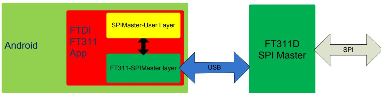
Figure 8.1 : Android FTDI FT311D SPI Master Application
