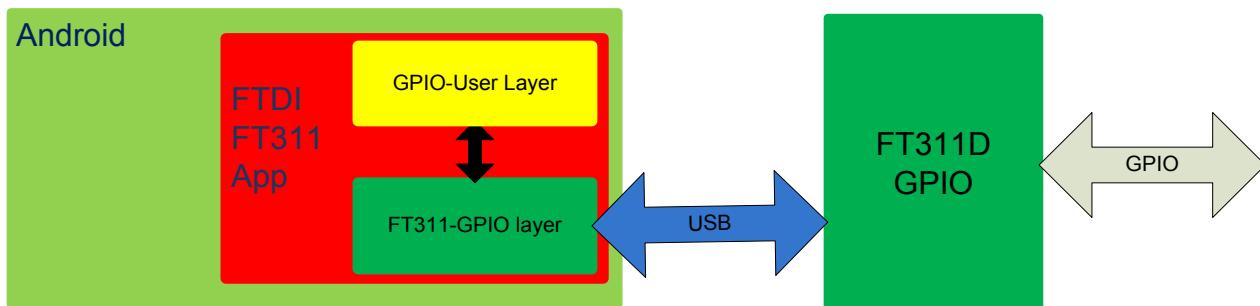
Figure 3.1 : Android FTDI FT311D GPIO Application
