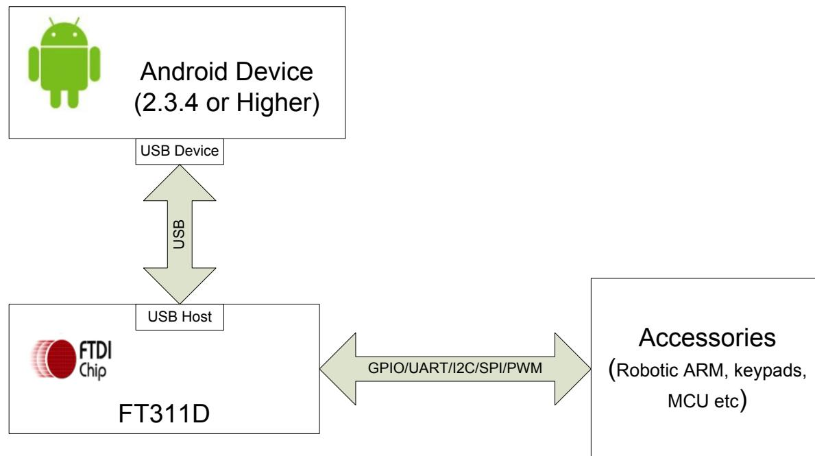
Figure 2.1 : Android Open Accessory Modules
