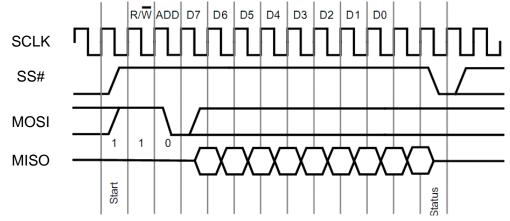
Figure 6.1 – VDrive2 SPI example
